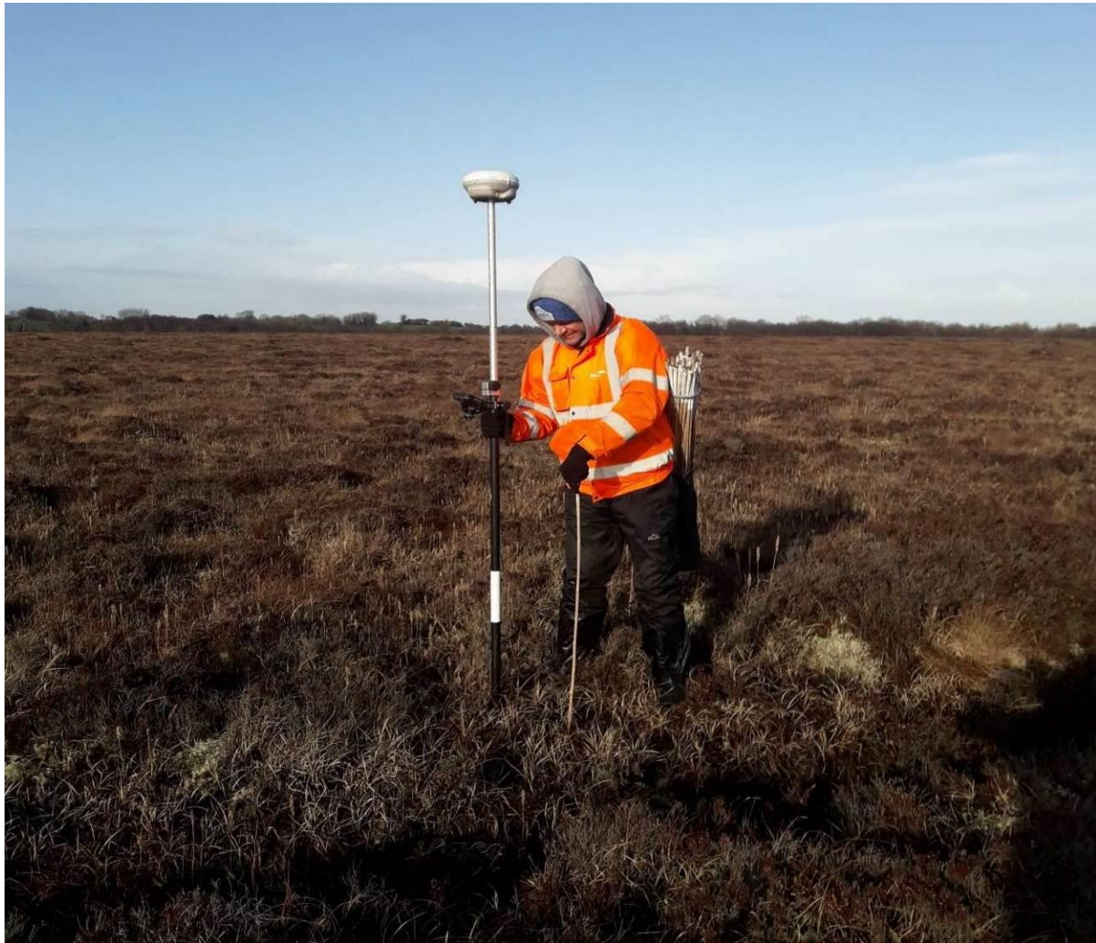
Figure 5.5 Example of Surveyor setting out on a high bog
