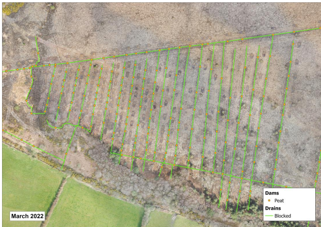
Figure 5.10 Post-Restoration ortho imagery at Ferbane Bog SAC
